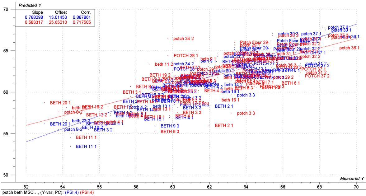
**Figure 3** Regression plot for the actual and predicted values for whole grain scanned with the Büchi instrument.
