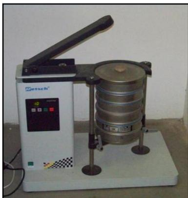
**Figure 1** The Retsch Rotap Sieve Shaker with duplicate sets of sieves.
