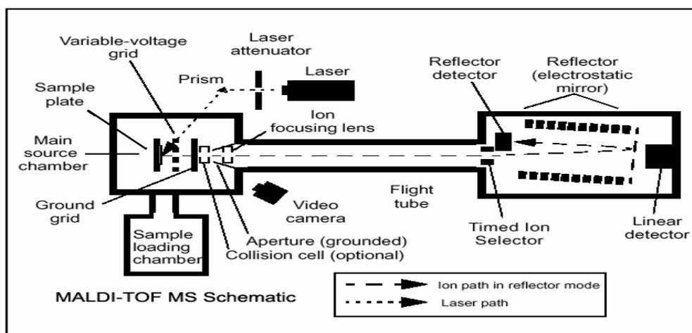
**Figure 3** Schematic layout of MALDI-ToF MS system.
