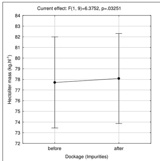
**Figure 2** Least square mean plot indicating differences between the HLM measurements before and after removal of dockage
