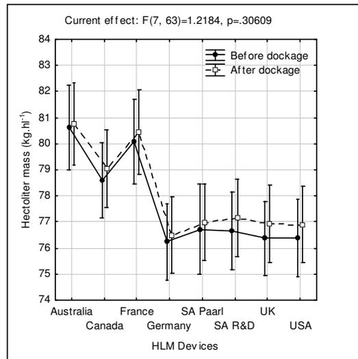
**Figure 3** Least square mean plot indicating no interaction between the HLM measurements obtained from the different hectoliter mass devices on maize samples before and after removal of dockage.
