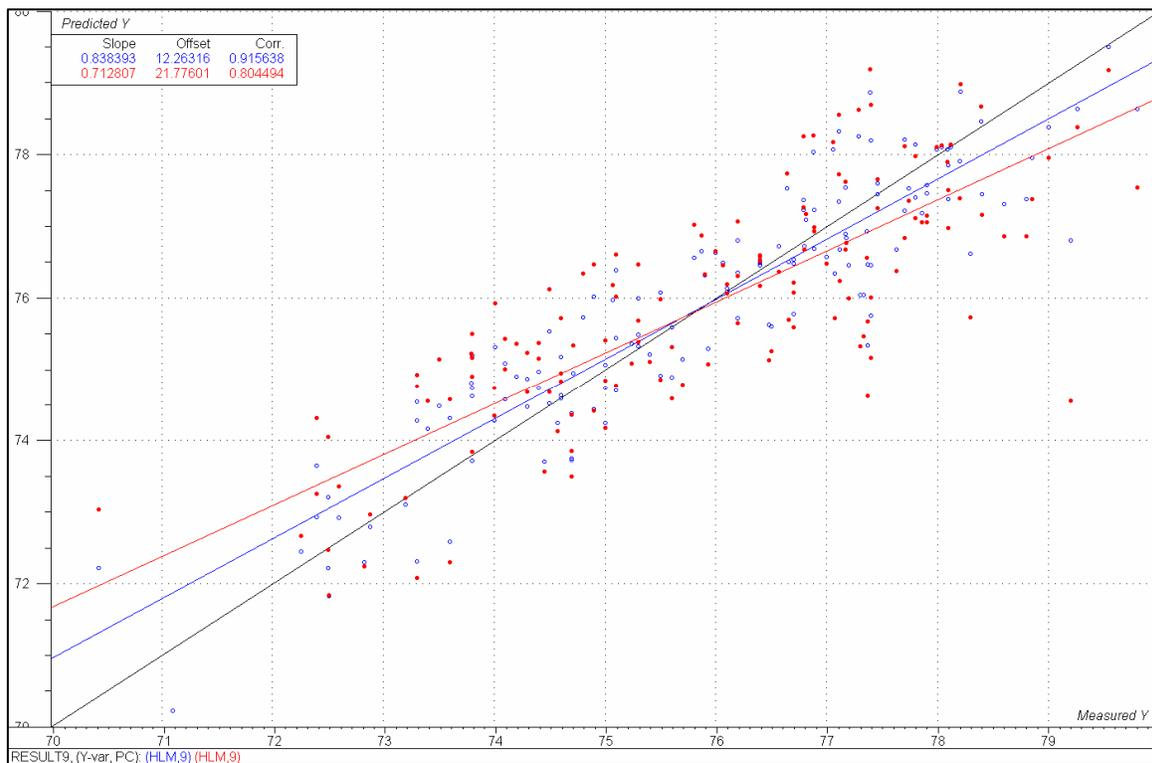
**Figure 4** Calibration (blue/open) and validation (red/solid) scatter plot of NIRS PLS calibration for predicting HLM determination of whole maize kernels using 9 PLS factors.
